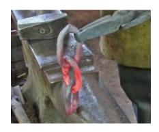
During my blacksmithing training, I took a rod and heated and pounded it, and dovetailed the ends, shaped the rod into an oval so that the ends were close together, heated it until it was bright yellow and then hit those ends together hard and fast so they fused. It's the ancient blacksmithing version of welding. And Bingo! After all that work I made a link. It tires me out to think about the energy needed to make a chain.
